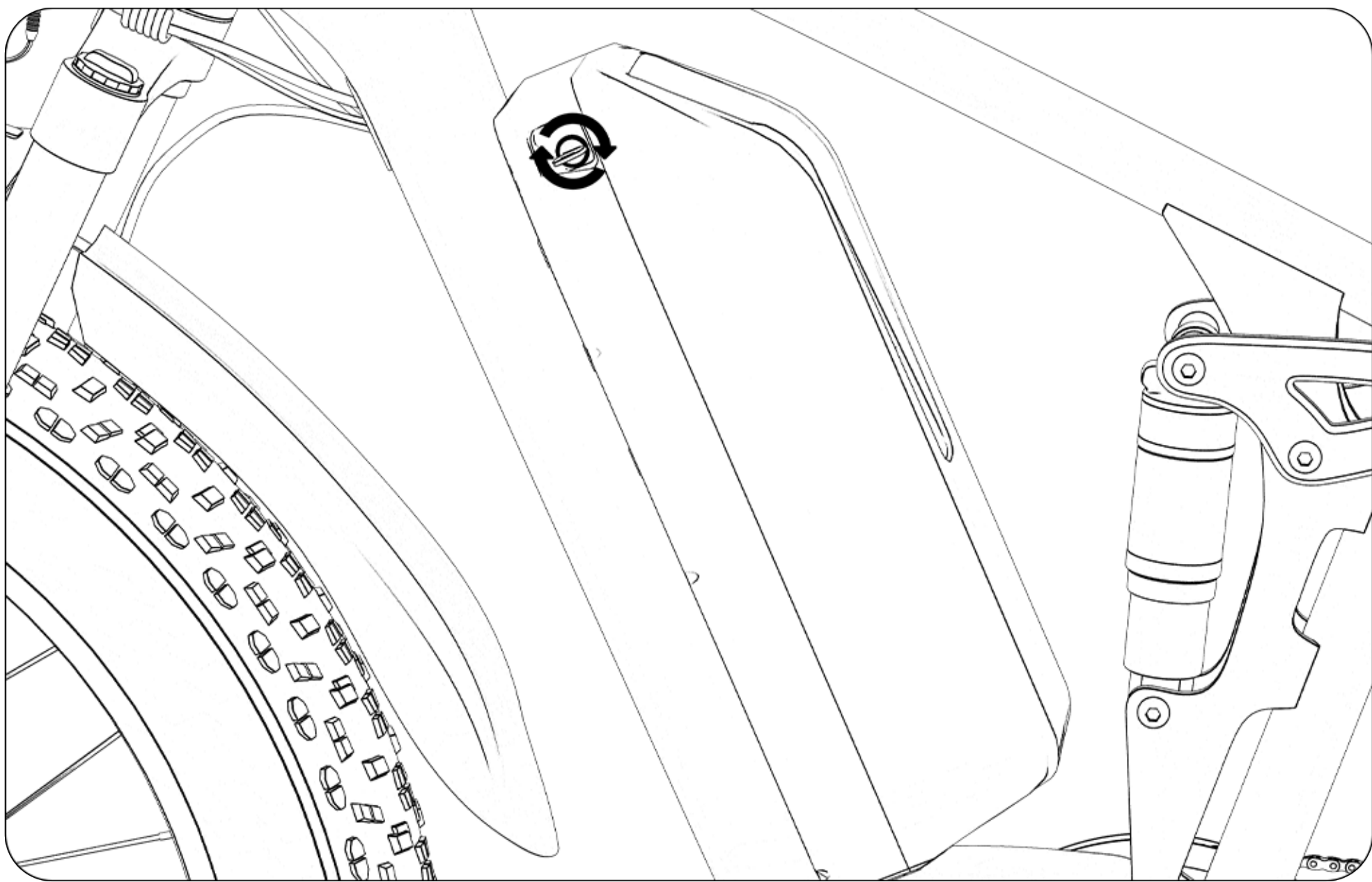
1. Unlock the battery with the key
