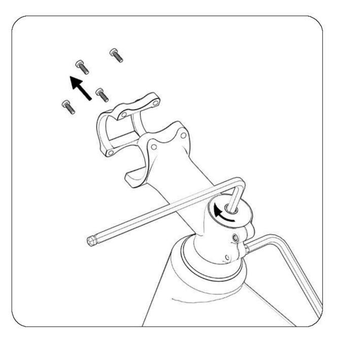
1. Adjust the Stem to the front and lock the screws with an Allen key. Use an Allen key to remove 4 bolts.
