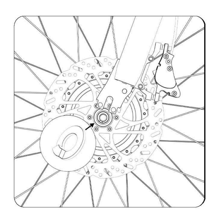
5. Place the spacer with the protrusion along the direction of the front fork, and then align the front fork with the motor shaft.
