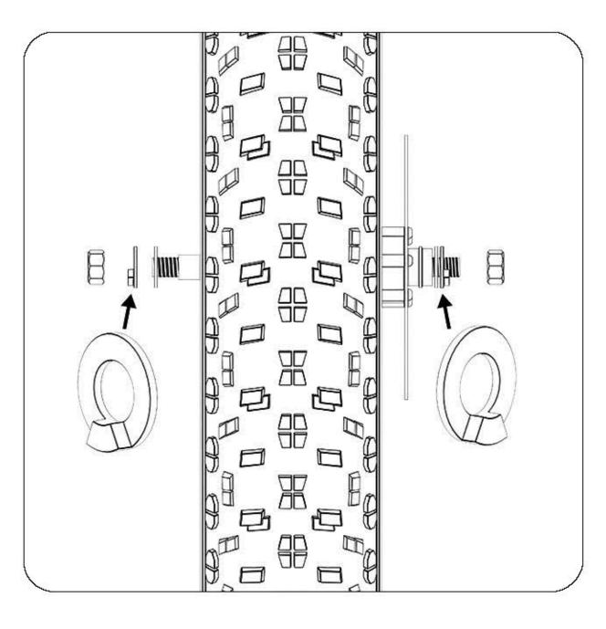
4. Place the gasket as shown in the picture with the raised side facing outwards.
