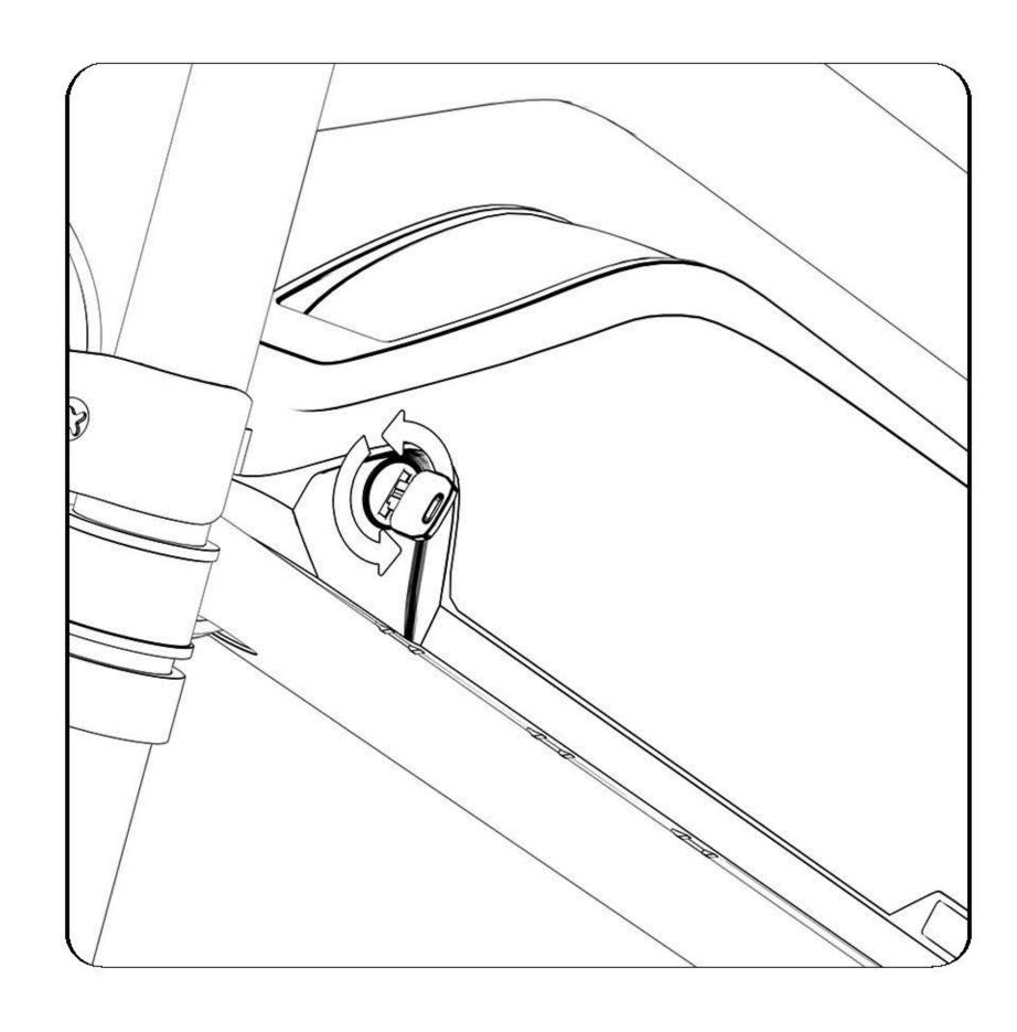
1. Unlock the battery with the key
