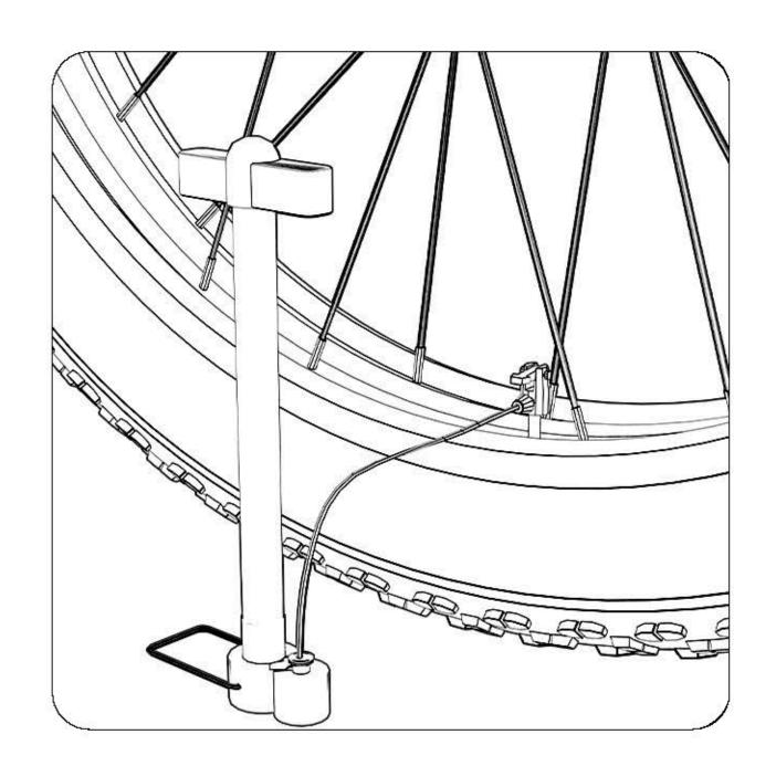
8. Inflate the front wheel slowly to prevent the tire from bulging out on both sides.
