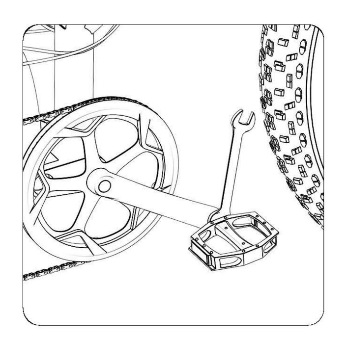
11. Use a wrench to tighten the pedal.
