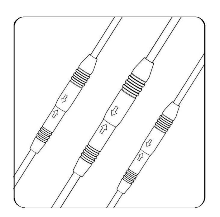
12. Connect the headlight cable, front wheel motor cable, and check the overall wiring.
