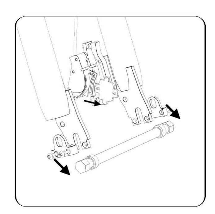
3. Remove the front wheel clip, then remove the front fork protection rod and brake protection pad.
