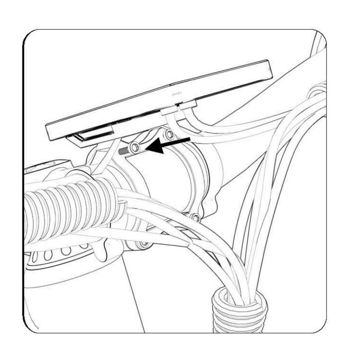
2. Attach the handlebar to the stem connection, and thread in the bolts.
