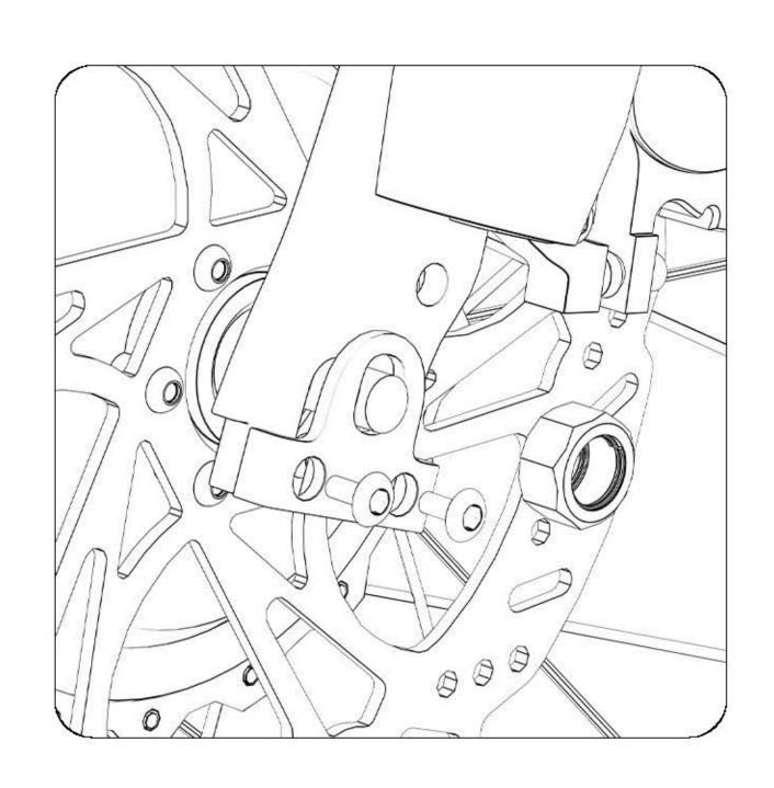
7. Install the front fork clip and tighten the screws, then tighten the screws with a wrench.
